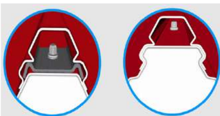
Screw cap for roof panel
